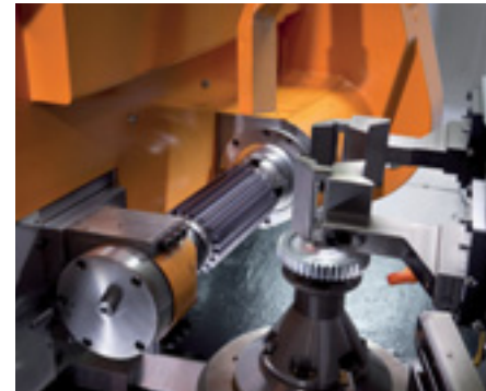
Automated gear cutting machine, production of gears
